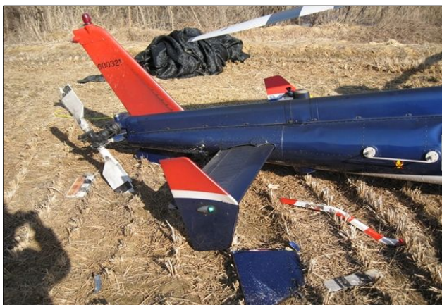
◀ [Figure 7] Damage to the tail rotor, the lower stabilizers and the tail skid
