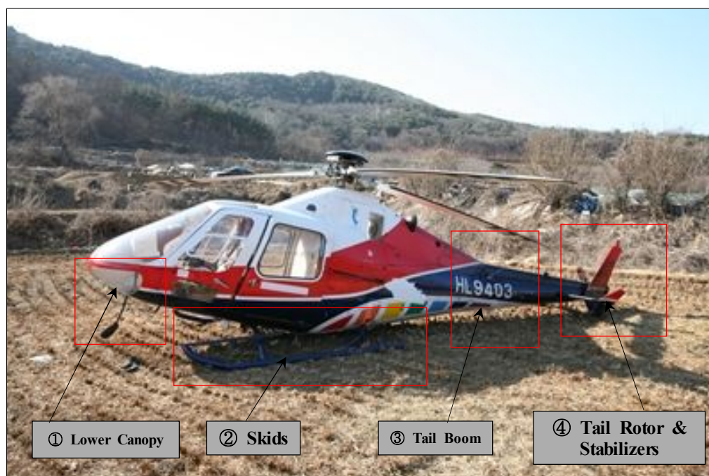
[Figure 3] HL9403 Major Sections of Damage
