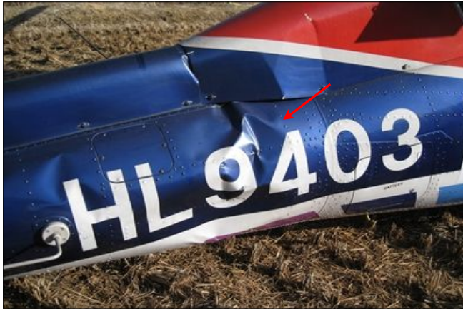
◀ [Figure 6] Tail Boom Wrinkle Caused When Bent Upward
