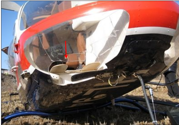
◀ [Figure 4] Damage to Lower Right Canopy (Red Arrow)
