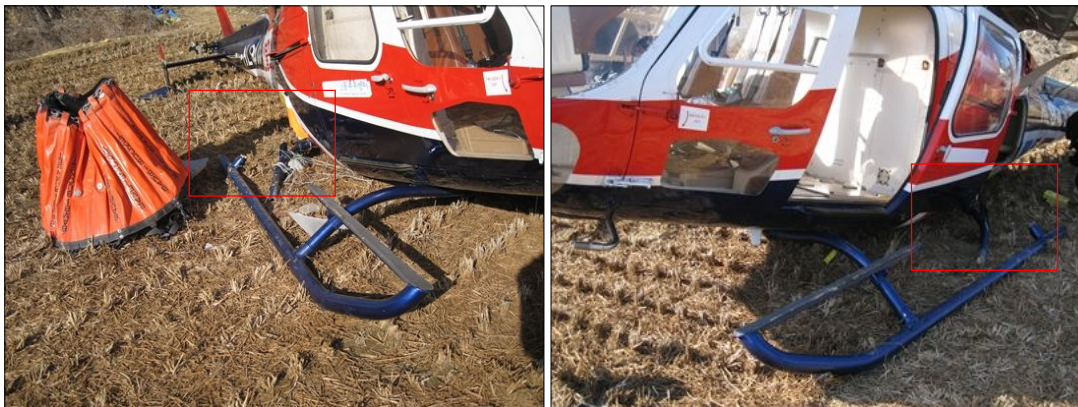
[Figure 5] Left & Right Side Skid Damage (Red Boxes)
